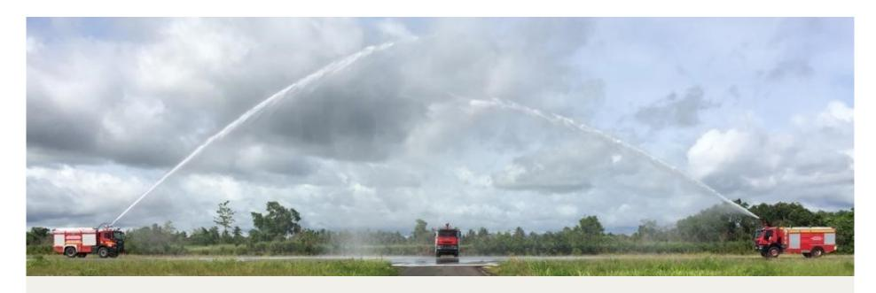
Fierre manufactures fire monitors specifically designed for vehicle installation. These fire monitors can be manual or electrical remote controlled such as the bumper and the roof monitor.
